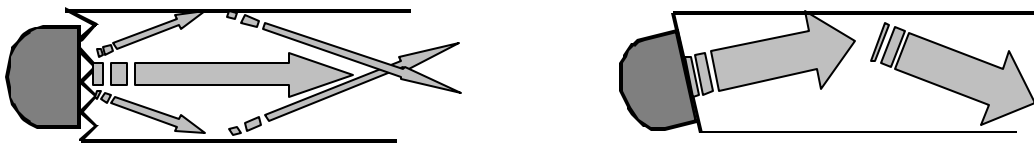
Figure 2 Rough and angled transducer contact
