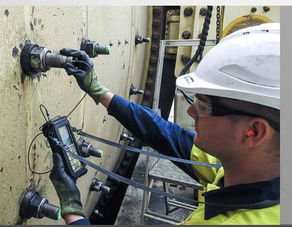
To eliminate instances of failure, each bolt is measured and adjusted to precise required bolt pre-load. Experienced NTS technicians complete the operation accurately and efficiently.
